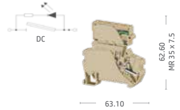
4 mm 2 Fuse Modular PushFit Feed Through Terminal Block 6.35x31.75 Fuse, 24 VDC with LED For 35 mm DIN Rail
