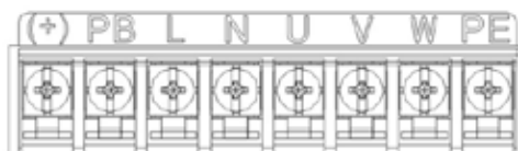
Figure 3-4: 1PH main circuit terminals (single phase)
