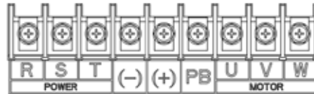
Figure 3-8: 3PH main circuit terminals (45-110kW)
